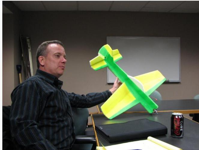
Rick Johnson brought his own design and scratch-built electric model. Made of EPP foam with carbon fiber reinforcement rods in the wings. Control is with elevator and ailerons only. A very light airplane that is fully aerobatic.
