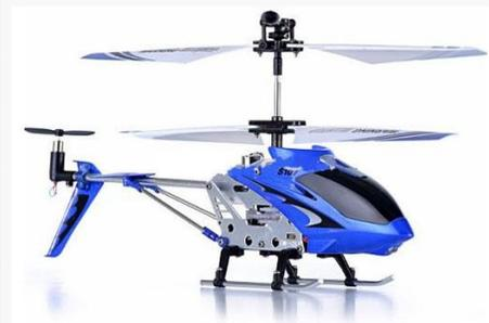
Picking up a bargain off the internet, **Bob Burt** found a micro chopper with transmitter for \$17.99 shipped. It has coaxial blades, and signal is transmitted by infra red. It has a 3.7v lipo battery that can be recharged through the transmitter or the USB port on your PC. Bob still needed to master the flying of this helicopter at the time of the meeting. But he thinks it was a good purchase and a quality built model. Note: This helicopter was available at NewEgg.com for \$22.50 shipped.
