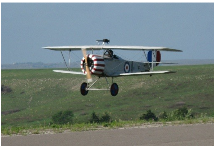
Tom Mahoney flying by with his 7/8 scale homebuilt Nieuport 17 powered by a Volkswagen engine.
